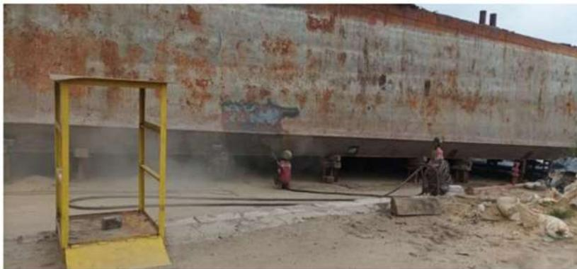
Gambar 4 Proses Sandblasting
