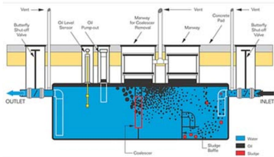
Gambar 2 Prinsip Kerja Oily Water Separator (Sumber: Ridwan, 2017: 5)
