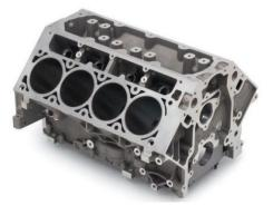
Gambar 6 Cylinder Block
