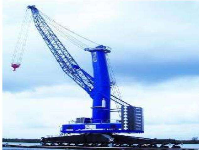
**Gambar 1 Harbour Mobile Crane (HMC)**
