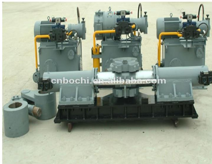
Gambar :2.1 Mesin Kemudi (wikipedia/steering gear2009)
