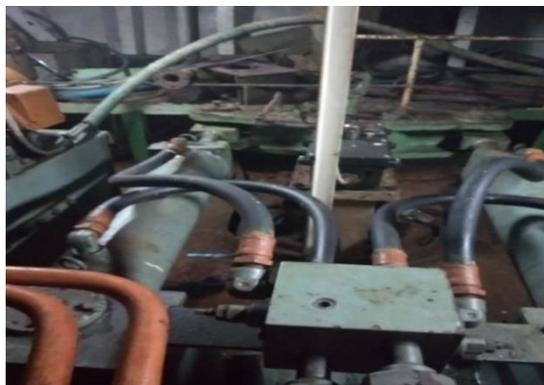
Gambar 8. *Steering Gear*
