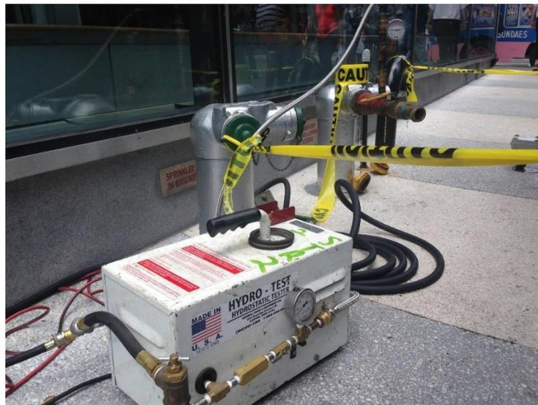
Gambar 3. *Hydrostatic Test*
