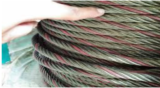
(Sumber : Stone Rd (2008). Anchor Windlasses) Gambar 2.7 Tali Kawat
