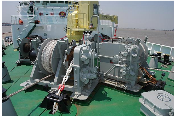
(Sumber : Lewmar (2017). Windlass and anchor operation basic safety ) Gambar2.10 Mesin Jangkar Tenaga Uap
