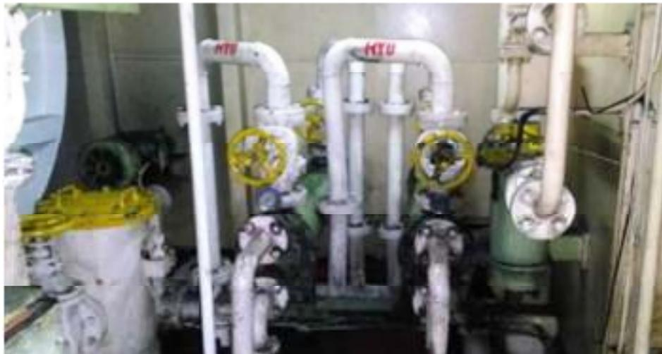
Gambar 2.9 Cooler Hydraulic Oil
