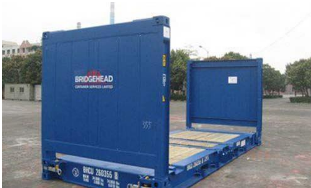
Gambar 6 Flat Rack Container
