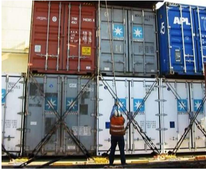
**Gambar 10. Kegiatan *Lashing/Unlashing* Pada Kapal Kontainer**
