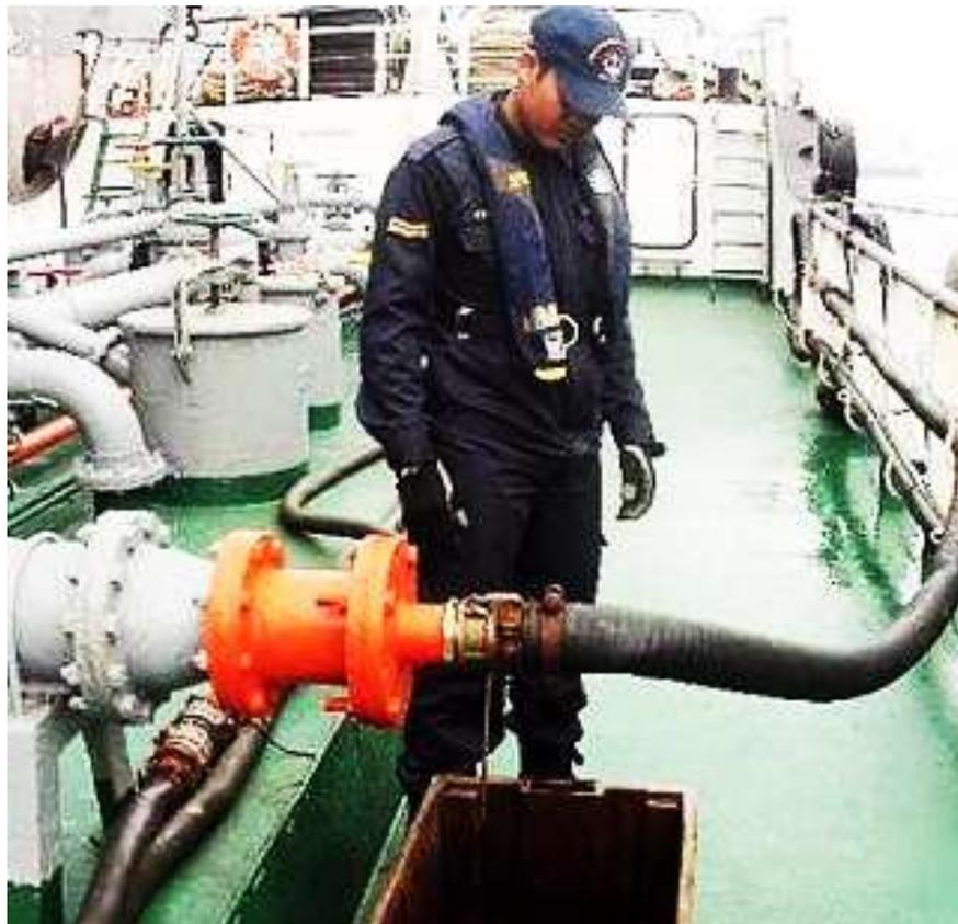
**Gambar 19. Pengisian MFO Dengan Metode Ship To Ship**
