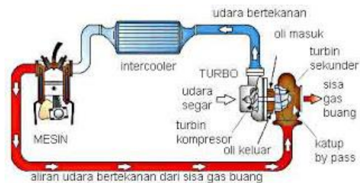
Gambar 10 Prinsip Kerja Turbocharger
