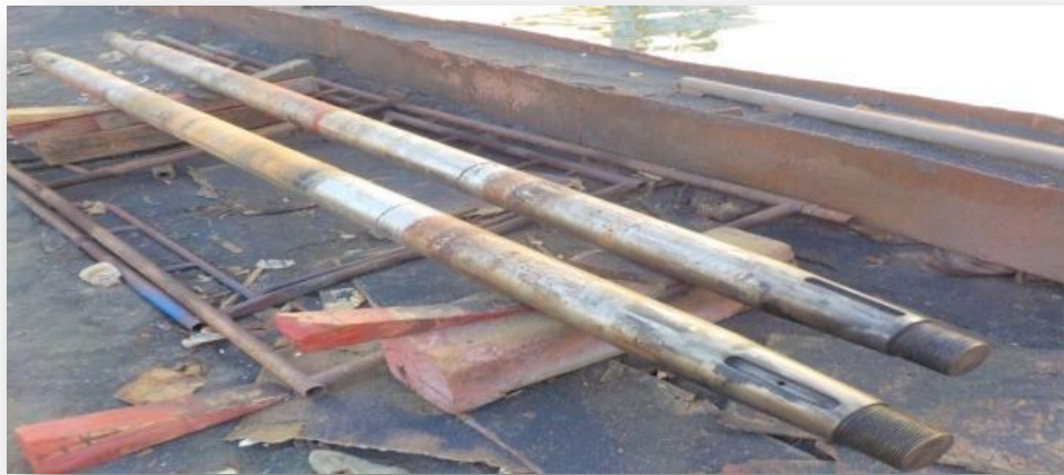
Gambar 5 pembersihan Propeller Shaft Sumber: https://IntermaditePropeller.com/auxiliary-engine.html
