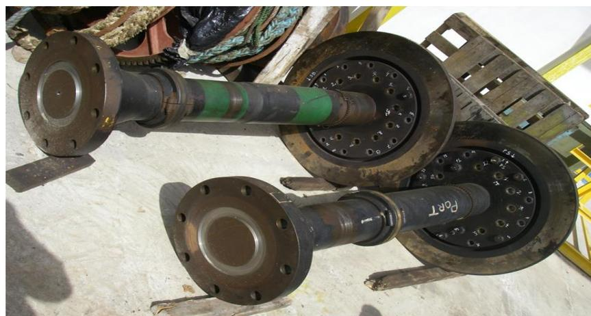
**Gambar 10** Poros Antara (*Intermediate Shaft*)
