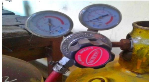
Gambar 8 Regulator *Acetylene Dock* Pelabuhan
