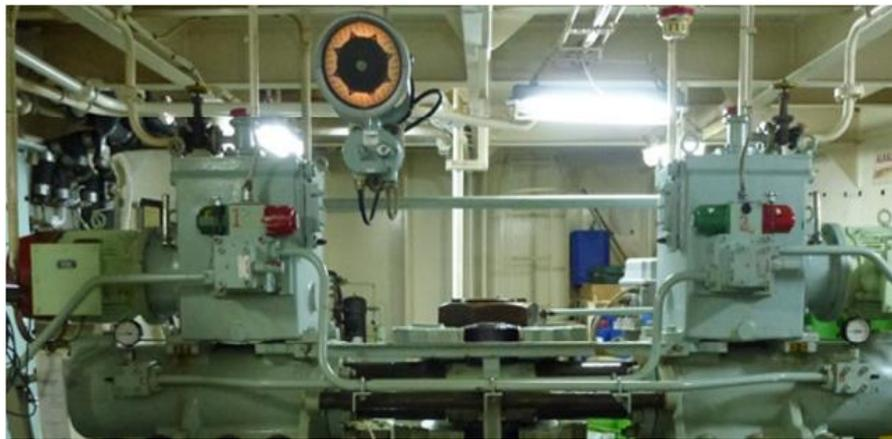
**Gambar 12** *Emergency Steering Gear*
