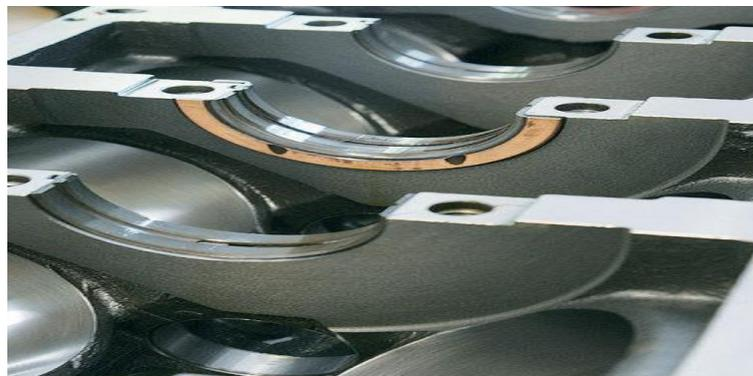
**Gambar 7.** Trust block bearing
