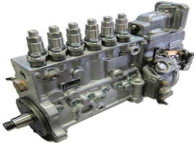
**Gambar 10.** Fuel injection pump
