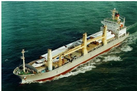
Gambar 3 *General Cargo Breakbulk Vessel*
