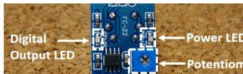
Gambar, 16 : *Digital Output LED*
