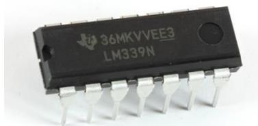
Gambar, 23 : *Voltage Comprator IC*
