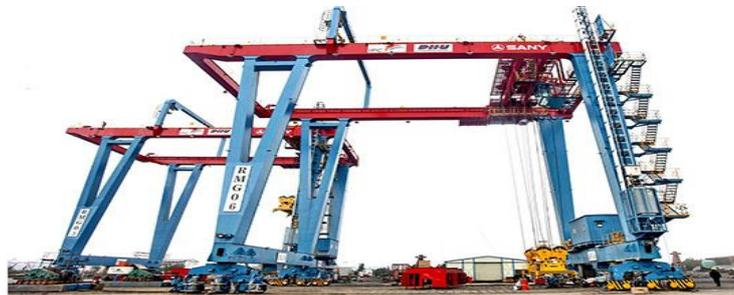
**Gambar 16. Rail Mounted Gantry Cranes**
