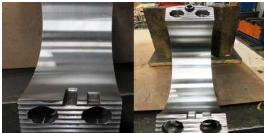
Gambar 2.3 connecting rod SV .MINERVA 88
