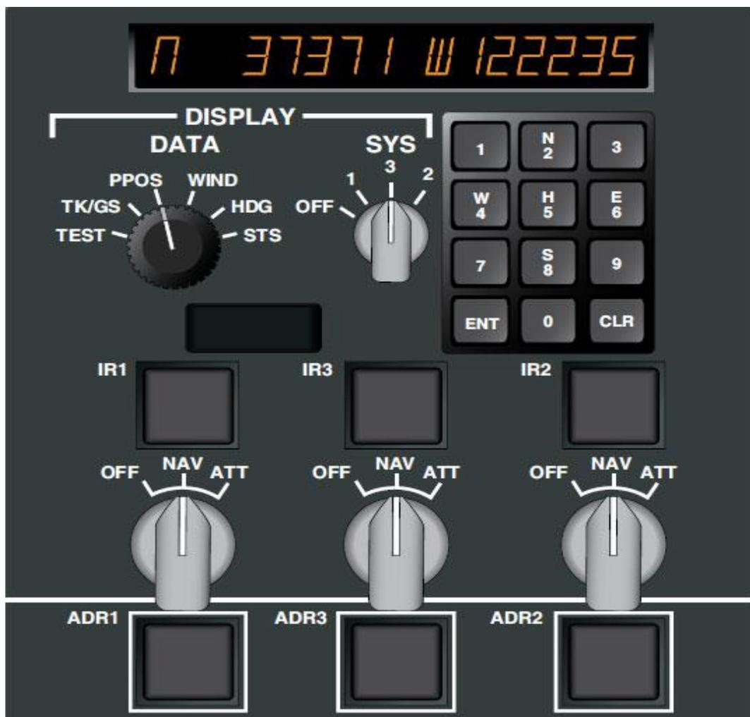
**Gambar 2.5 :** *Inertial Reference System*
