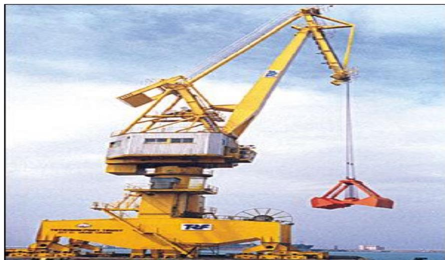
**Gambar 5 *Level Luffing Gantry Crane (LLGC)***
