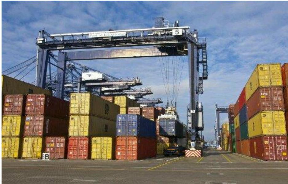
**Gambar 4 RTG (*Rubber Tyred Gantry*)**
