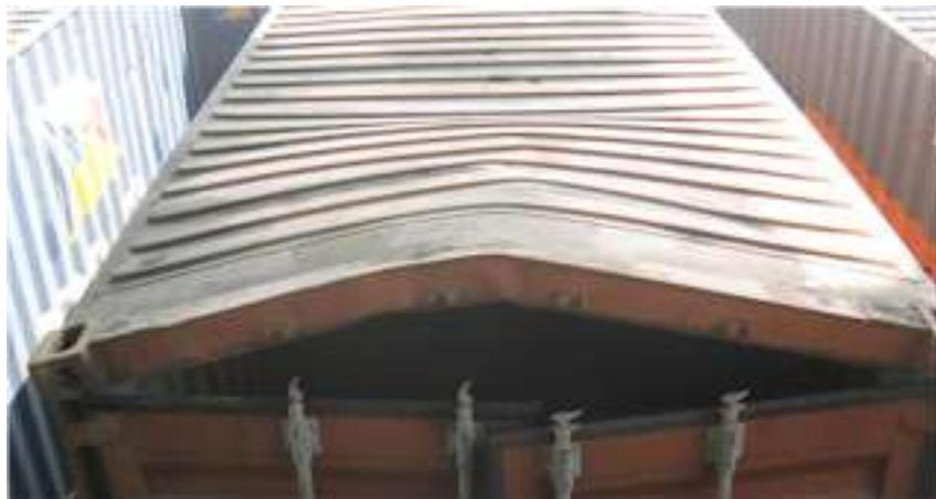
Gambar 2.1 *damage container*
