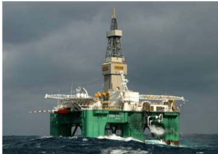
Gambar 3 Semi-submersible platform Sumber : Offshore Utility
