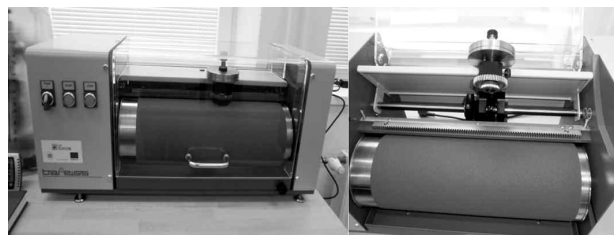
Figure 1. Testing device for determination of abrasion resistance
