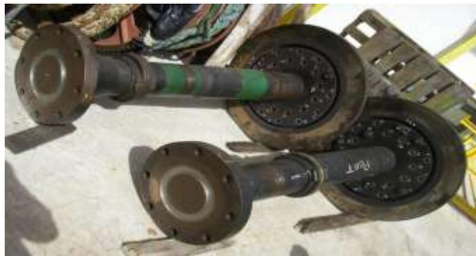
Gambar 12 : Poros Antara (*Intermediate Shaft*)
