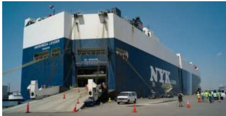
Gambar 6 Stern ramp door. Sumber :
