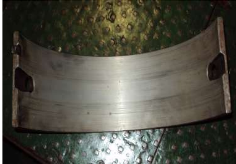
Gambar 8 Keausan main bearing (Dokumentasi: 19 September 2019)
