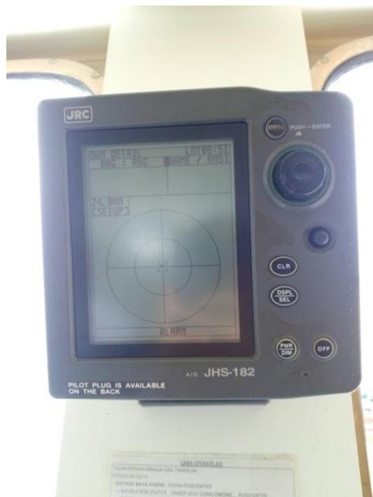
Gambar 2.4 (AIS *Automatic Identification System*)
