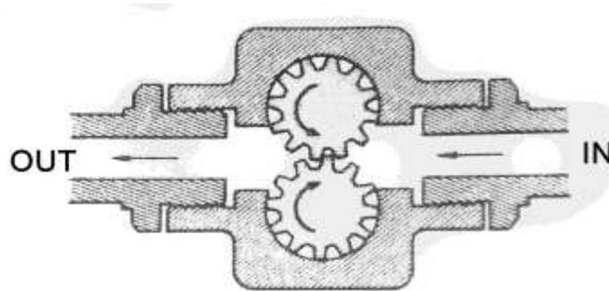
**Gambar 9.** Gear pump
