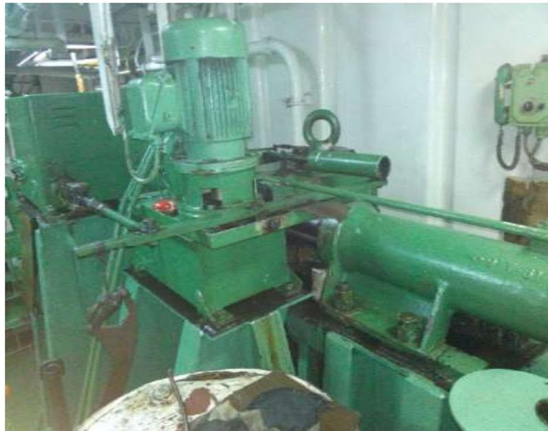
Gambar 2.1 Electro Hidrolik Steering Gear.
