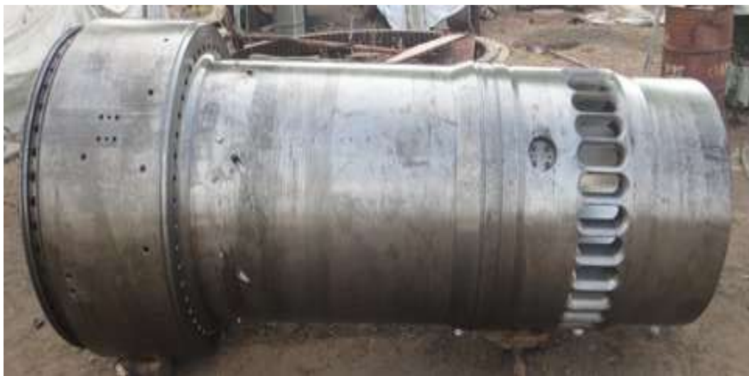
Gambar 5 Cylinder Liner KM. Meratus Tangguh 2
