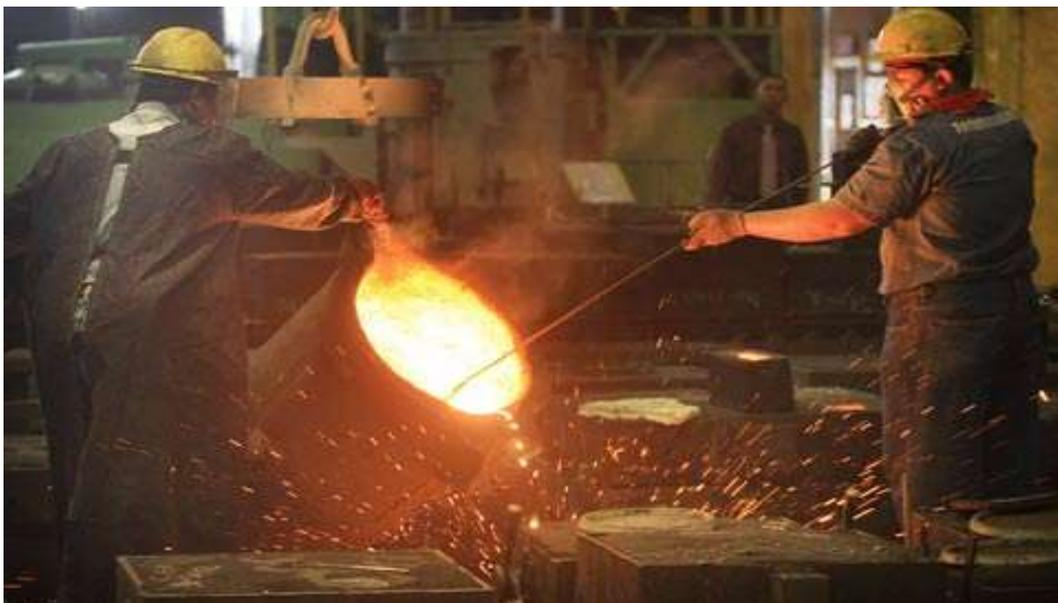
**Gambar 2.2. Proses Pengecoran *Cylinder Head***
