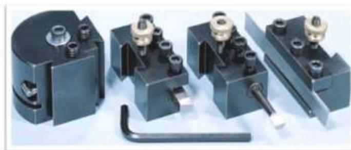
Gambar 8. Pemegang Pahat Dapat disetel (Adjustable Tool Post)
