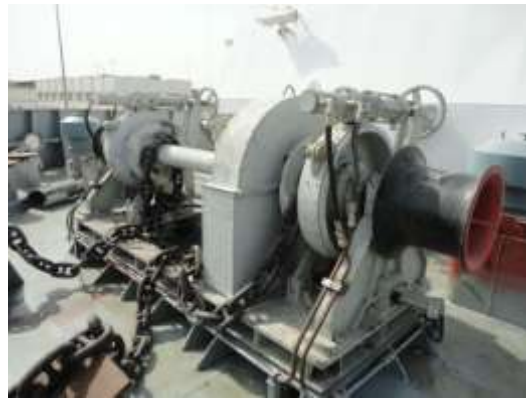
Gambar 2.9 wind lass berporos horizontal
