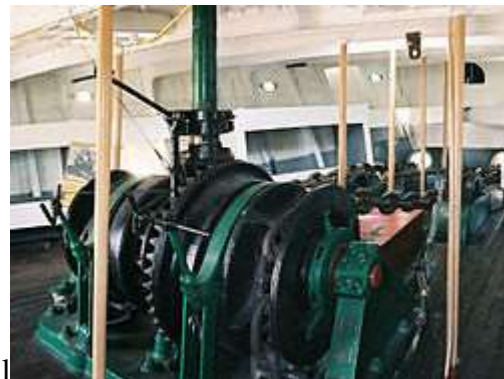
gambar 2.10 wind lass berporos horizontal
