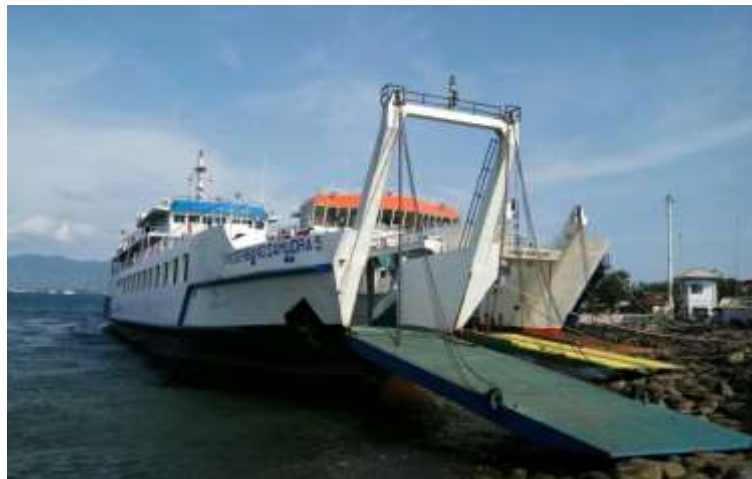
Gambar 3 Pintu Rampa Kapal Gerbang Samudra Sumber: PT Gerbang Samudra Surabaya, Kmp. Gerbang Samudra 5 Surabaya
