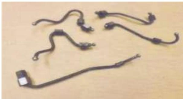
Gambar 3. Over Flow Pipe
