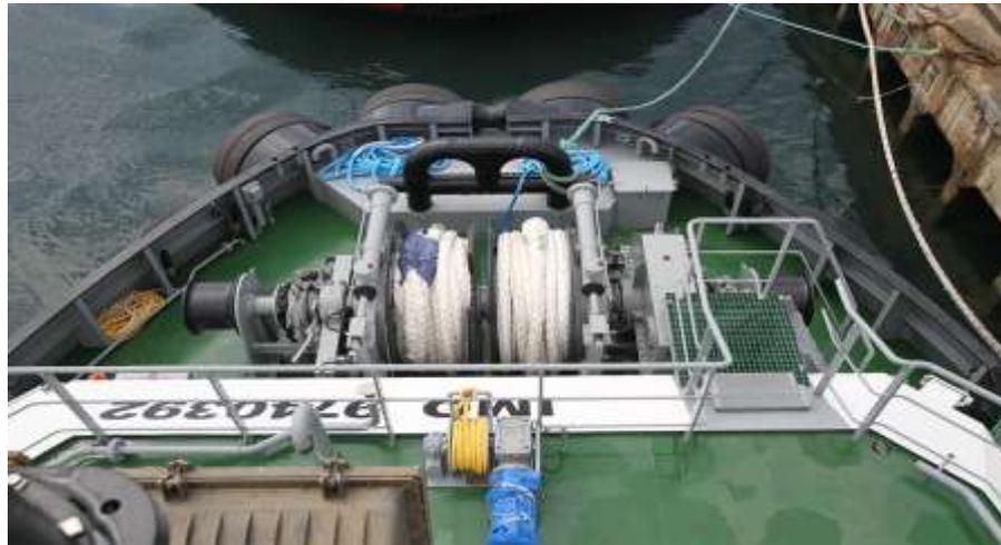
Gambar 4 Mesin *Windlass* dikapal KN. SAR SADEWA 231
