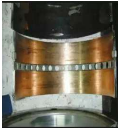
Gambar 2.16. Bearing/metal KMP.GERBANG SAMUDRA 3
