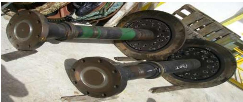
**Gambar 11 : Poros Antara (*Intermediate Shaft*)**
