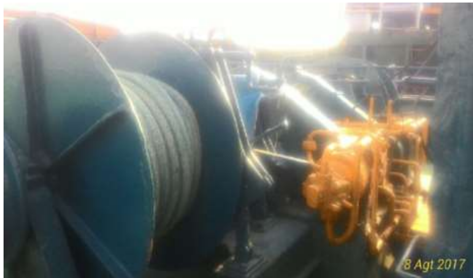
Gambar 2.2 Mesin windlass penggerak electro hydraulic
