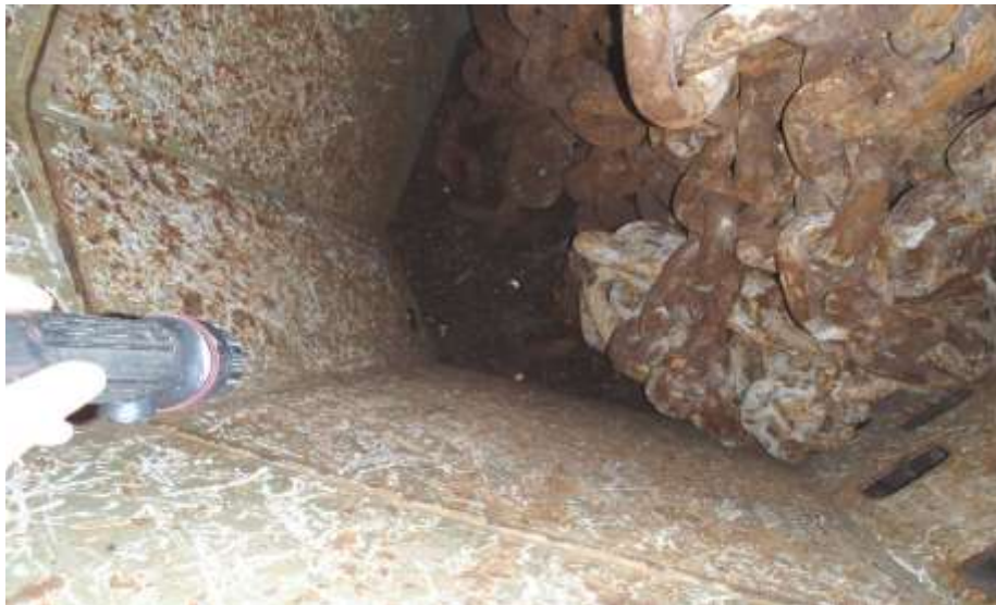
Gambar 2.8 Bak Rantai Jangkar anchor chain locker di Kapal MV. JK GALAXY PT. AMAS SAMUDRA JAYA
