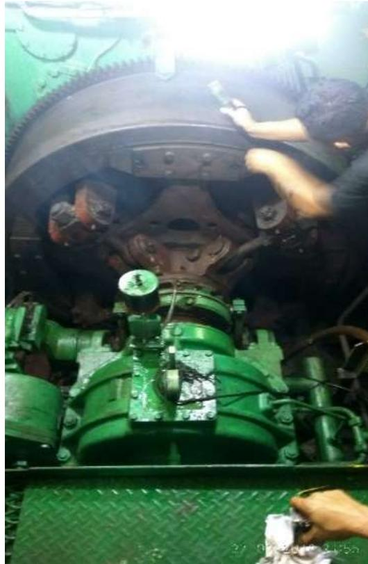
Gambar 2.5 Intermediate shaft Propeller
