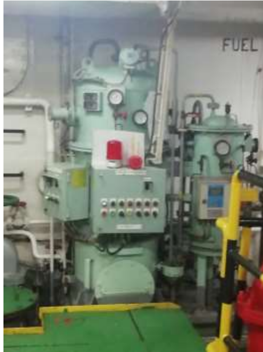
Gambar 1 Fresh Water Generator Sumber : Manual Book Survey Ship Barakuda
