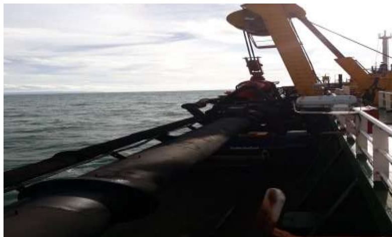
Gambar 8 : Ladder TSHD. King Arthur 3
