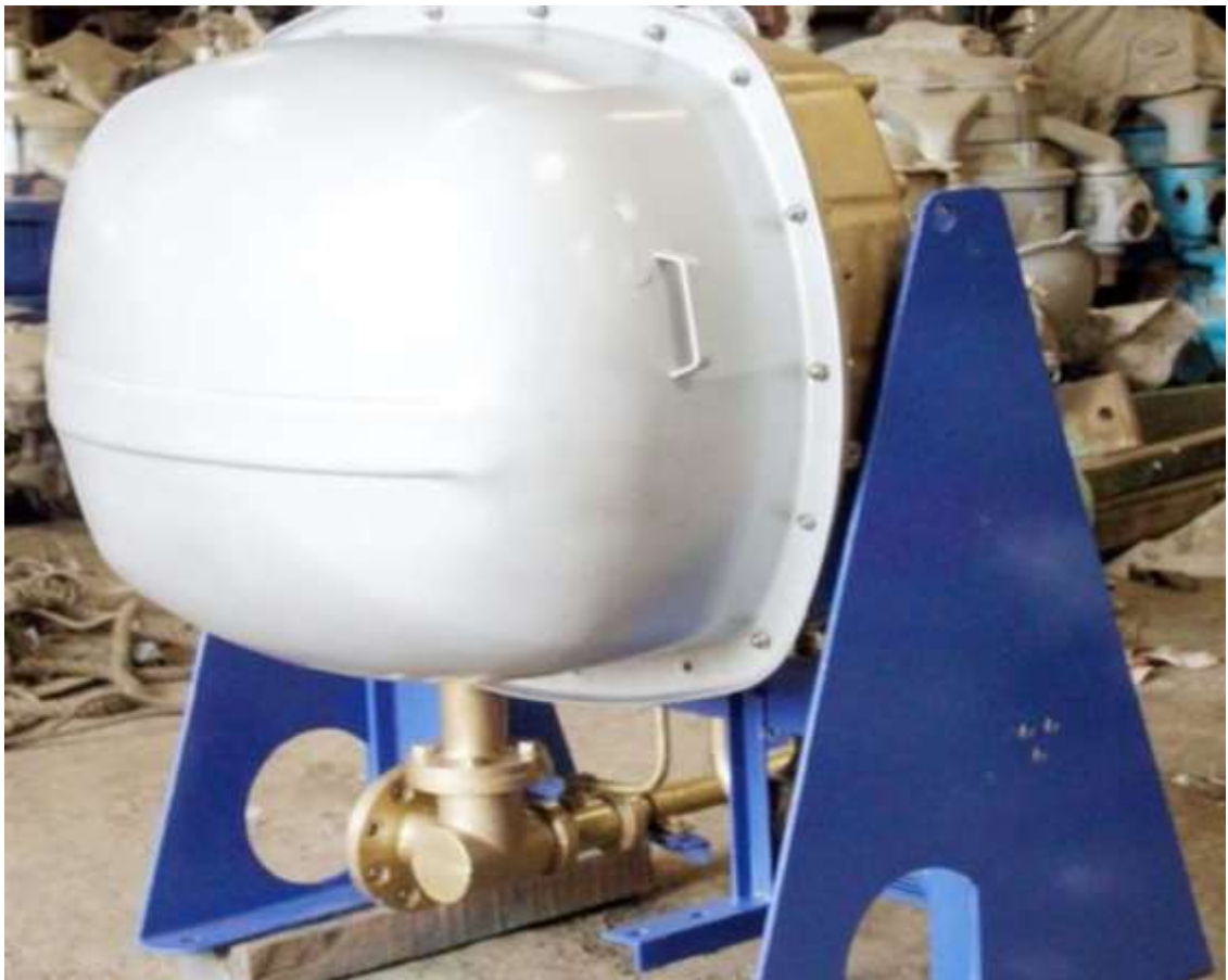
Gambar 5 Fresh Water Generator
