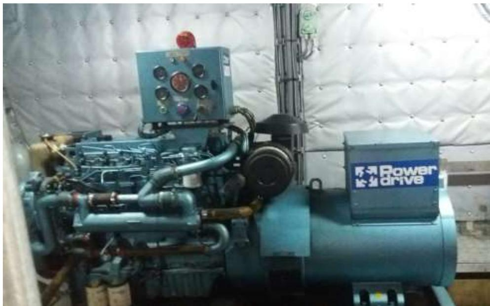
Gambar 1 Gambar Generator Kapal
