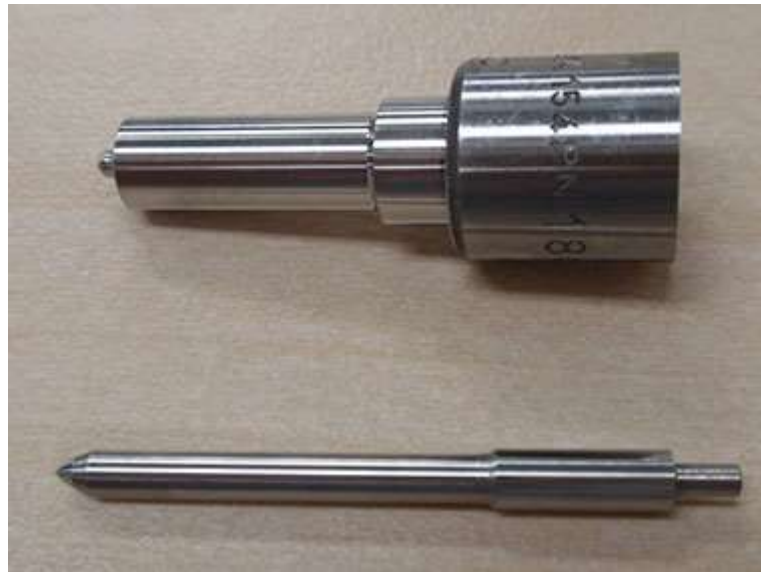
Gambar 8 : Nozzle needle (Widopo Cahyo 2016 Komponen Injector Diesel )
