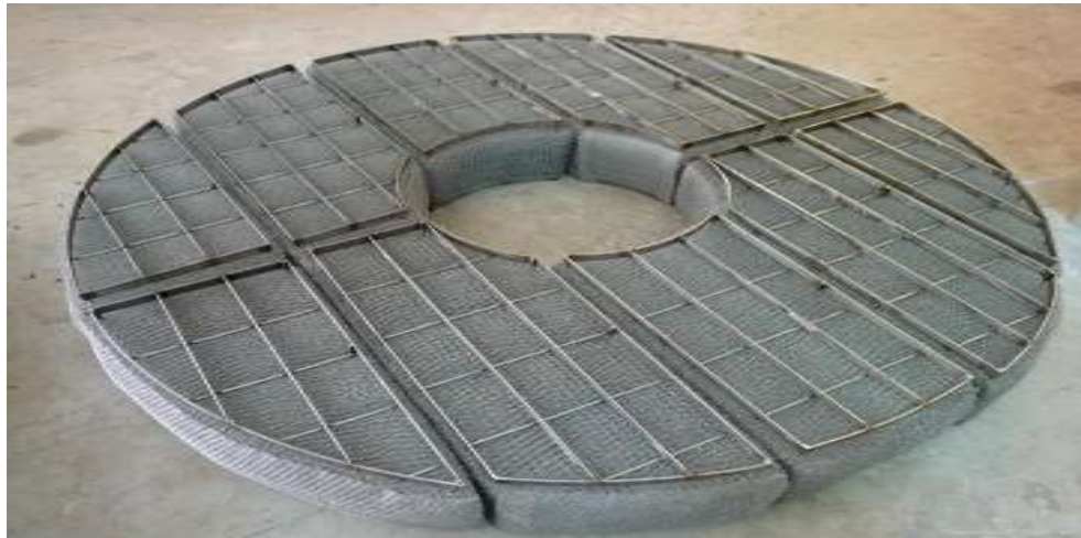
Gambar 13 Demister of Fresh Water Generator
