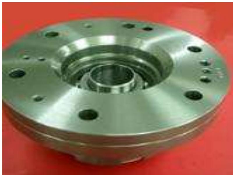
Gambar 2.4. Bearing Turbocharger
